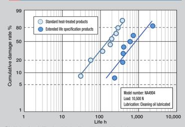
This table shows the result of life testing under load conditions at 50% of the basic dynamic rating. The Extended Life specification with special heat treatment lasted 5 times longer or more in L10 life compared to the standard heat-treated products
